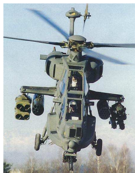
Agusta A129 attack helicopter, with rocket pods, Hellfire launchers on port side, and TOW launchers on starboard side.
